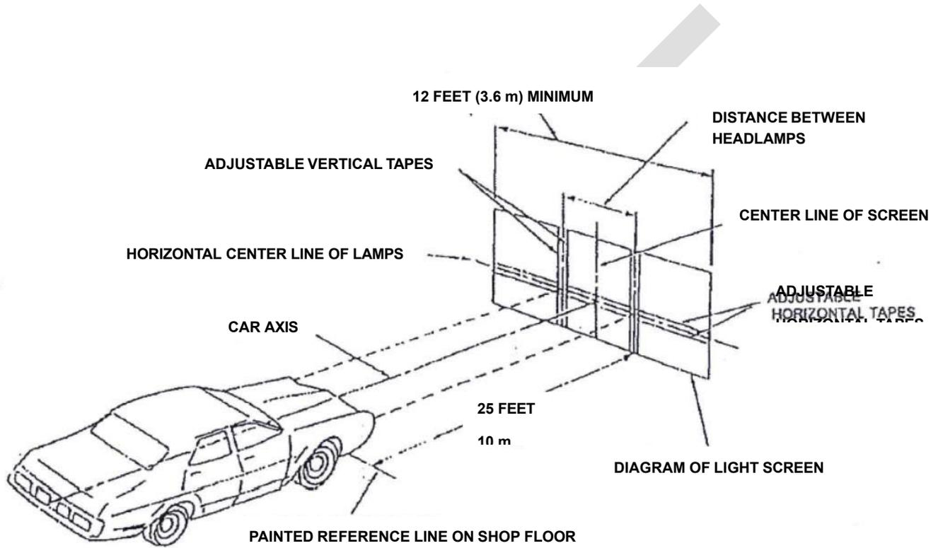
Figure D.2 Irradiating range of headlights
